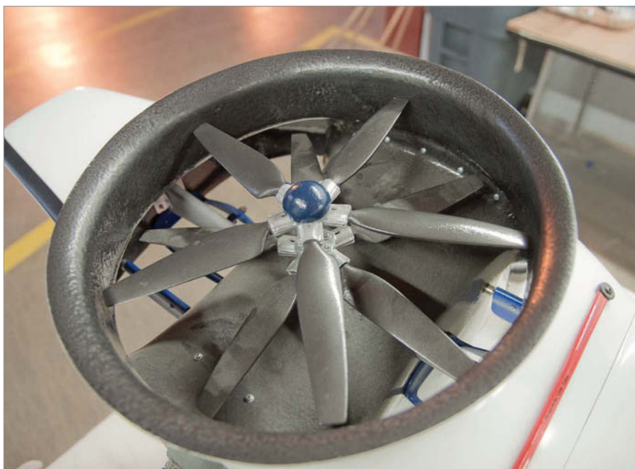
Top view of the counter rotating blades. There are two, five-bladed hub assemblies and a cone-shaped spinner cap.
