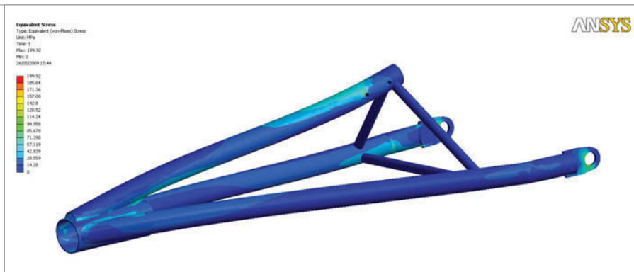
This is an ANSYS simulation of the stress distribution in the Ocean Treader arm.
